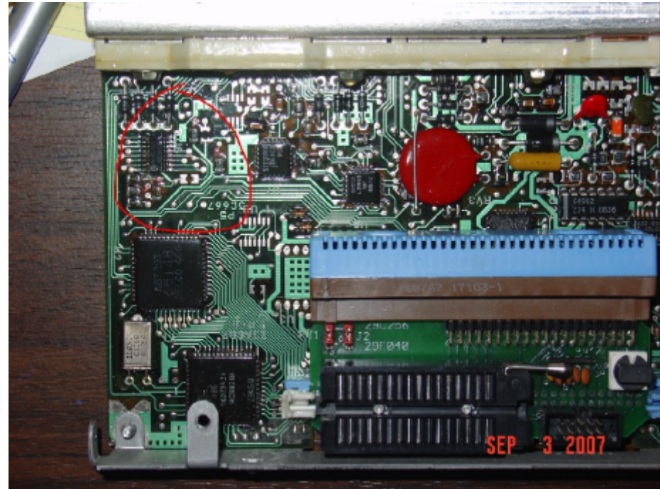
Location of the U6 chip and its input resistors
